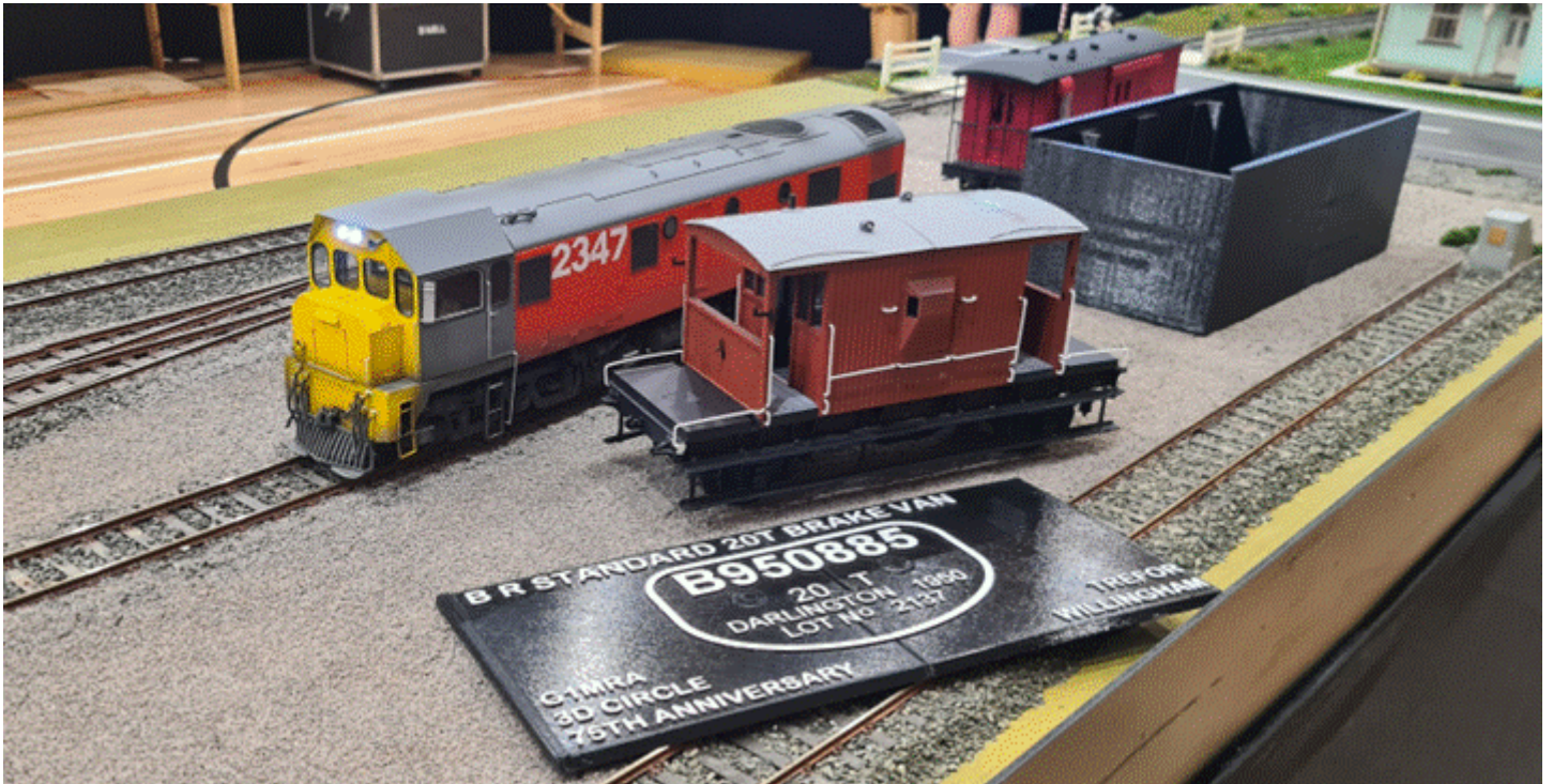
A rebuilt DG class locomotive with a hood cab added. The original cabs were notoriously prone to leaks from wind and rain and were hardly weatherproof. Originally built by English Electric, these did not last nearly as long as their GM counterparts and had all gone by the early eighties. Note the typical NZR brake van in the background as a comparison.
