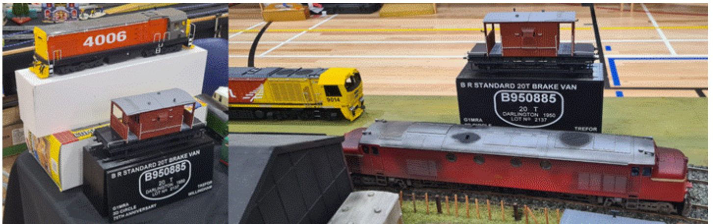
Moving up a scale, this is the work of the NZR 9mm to the foot group. This scales out at roughly 1:33 which is close enough to the 1:32 of the brake van. Thus, in size they are reasonably comparable. Of course, the scale is set to allow the use of O gauge track to represent the NZR 3' 6" standard gauge. Narrow gauge this is not! Of particular interest is the loco on the left (NZR DC class) which is 3-D printed. The loco prominent on the right is an original English Electric DF built in the mid-fifties as a precursor to the BR class 40s and 37s.
