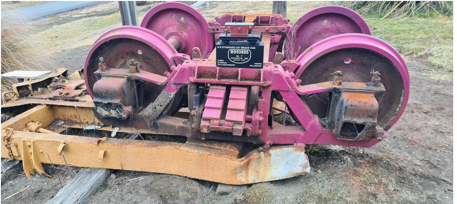
A bogie and undercarriage section.
