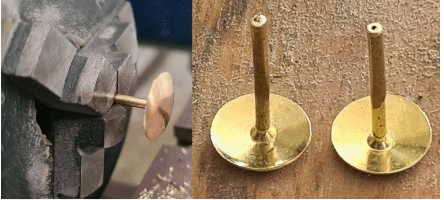
The prepared buffer heads. N.B. Brass drawing pins make great wagon buffer heads.
