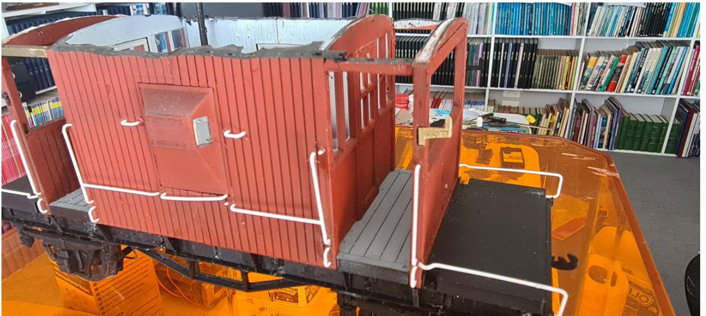
One of the enhancements made, was to fit glazing to the windows which had previously been open. Note also the damaged handrails which are likewise plastic. If I had more time I would have made up metal rails but since I was on a deadline, I simply glued the rails back in place. Maybe a job for the future. Note also the brass lamp iron on the top right where one of the plastic originals had gone AWOL.
