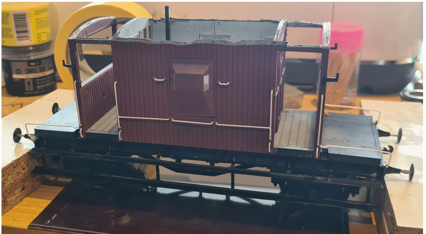
One of the footsteps glued in place and likewise, the buffers. The buffers are being supported by the wooden blocks on either side of the van whilst the glue sets.
