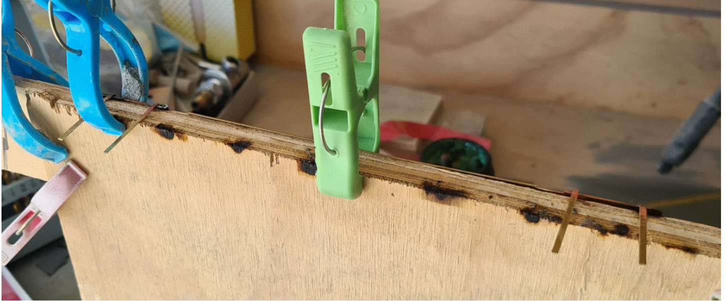
Connecting straps being soldered in place.
