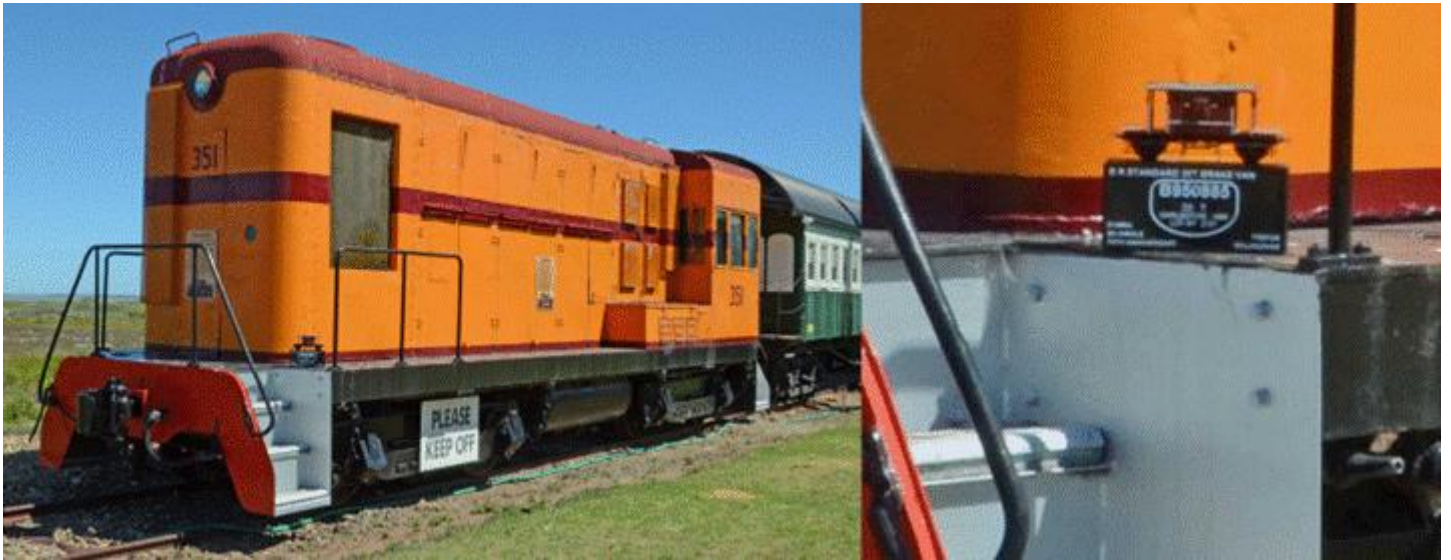
BV on SAR English Electric powered 5' 3" gauge shunter 351 built 1949 seen at the same location.
